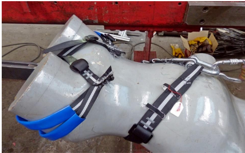
Figure 20 - Failure of safety stitching during the harness strength test
