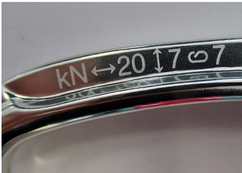
Figure 11 - Example of marking of guaranteed strength values on a connector
