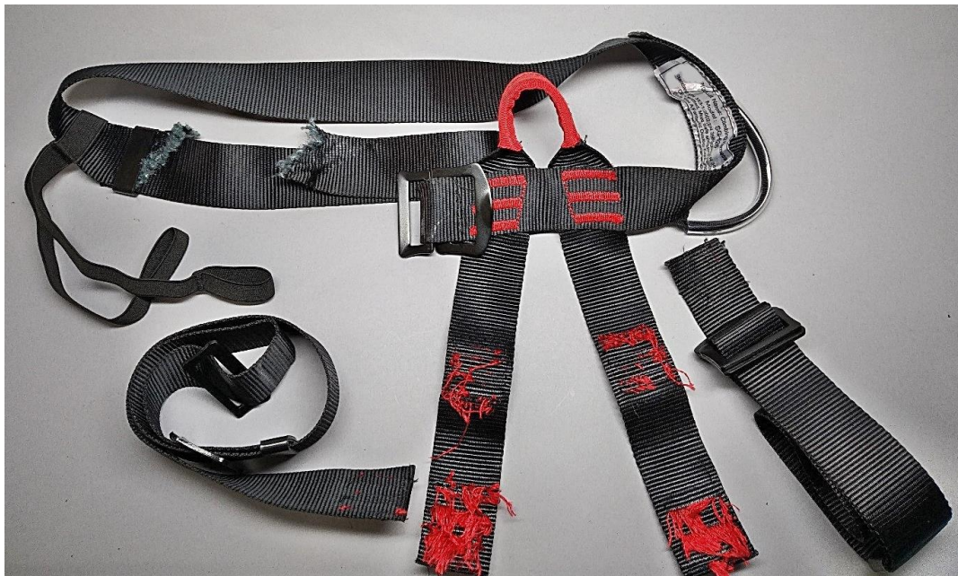
Figure 19 - Harness torn during the harness strength test
