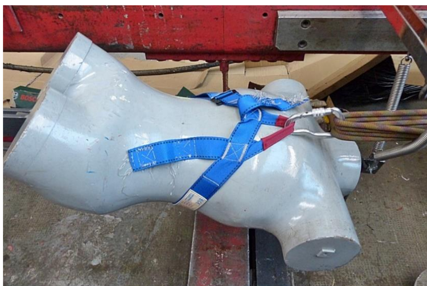
Figure 17 - Harness torn during the harness strength test
