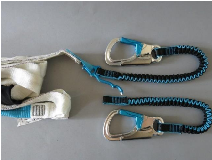
Figure 22 - Breakage of the secure resting connection of an EAS during the static test
