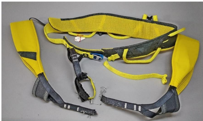
Figure 21 - Harness torn during the harness strength test
