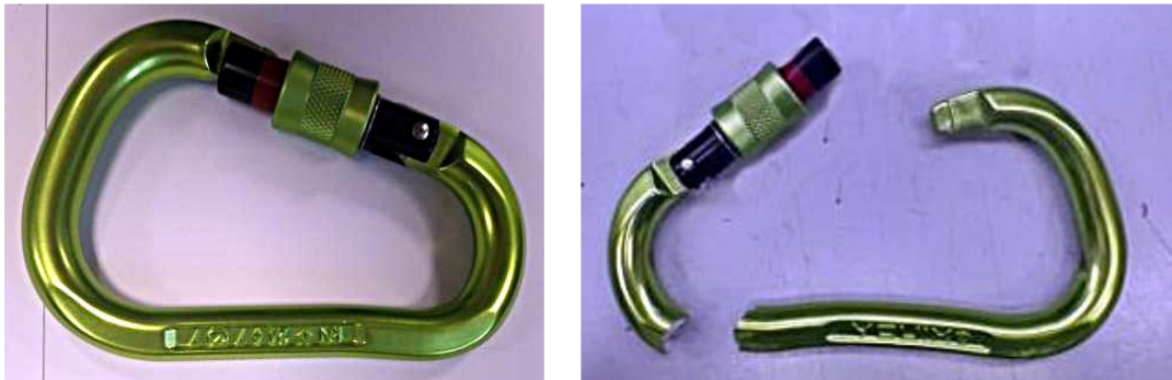
Figure 10 - Basic connector before and after a strength test
