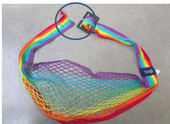
Picture 7: Failure for 8.5 Durability The carrier breaks
