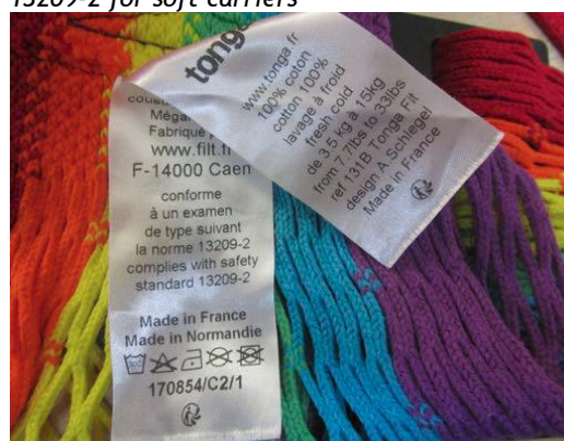
Picture 8: Failure for 10.3 Marking The sling is marked as compliant to EN 13209-2 for soft carriers
