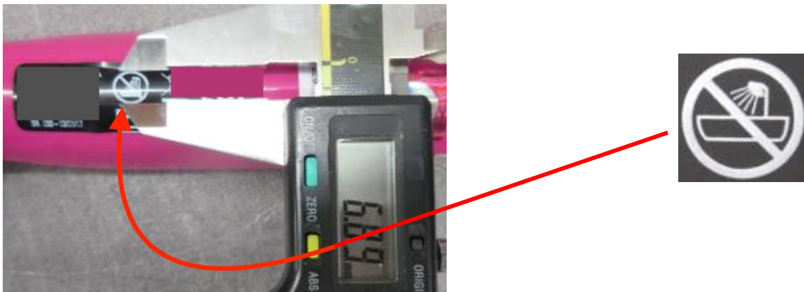
Figure 8 Undersized warning symbol
