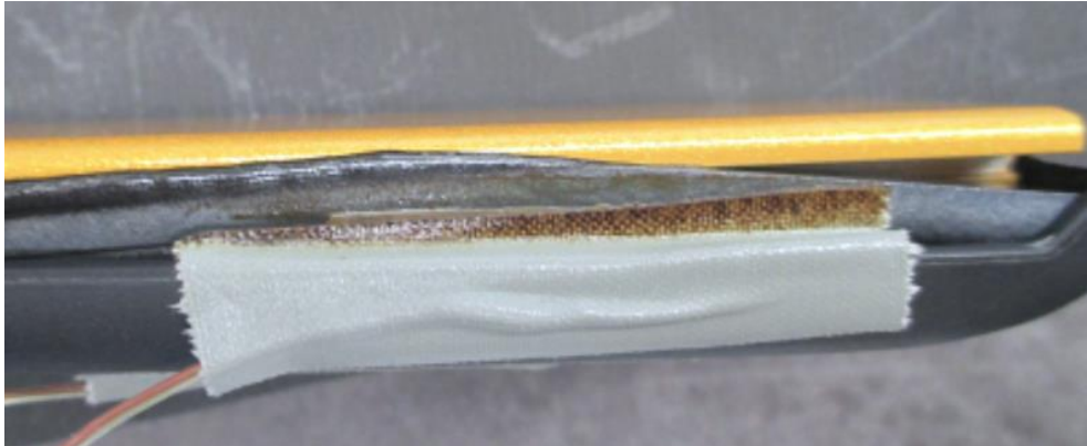
Figure 14 Enclosure deformation after abnormal operation test
