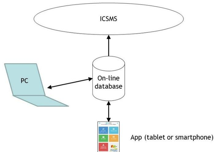
Figure 1: Structure of MSTyr15 data collection system
