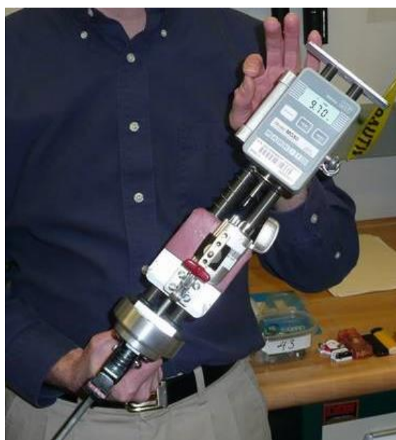
Figure 6. Test probe designed by CPSC for indicative on site measurements of the child-resistance of lighters of the hard-piezo pusher force type.
