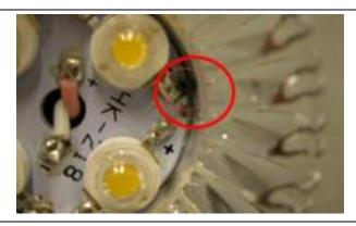
RESISTANCE TO FLAME AND IGNITION parts of insulating material subjected to the glowwire test of 650  $^{\circ}\text{C}$
