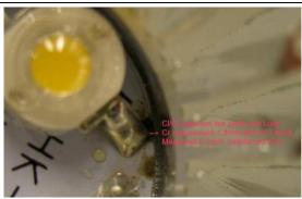
FIXING OF CONDUCTORS checking the fixing of the conductors on the PCB of LED lamp control gear
