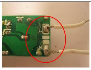
Figure 3 - Main defects found during tests
