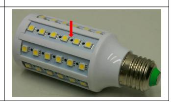
INSULATION RESISTANCE AND ELECTRIC STRENGTH tests between live part and accessible parts
