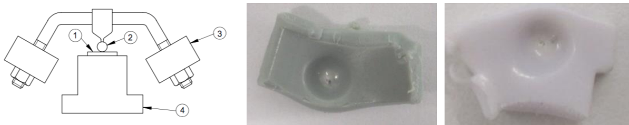
Figure 16 Ball pressure apparatus and indentation in samples exceeding 2 mm in diameter
