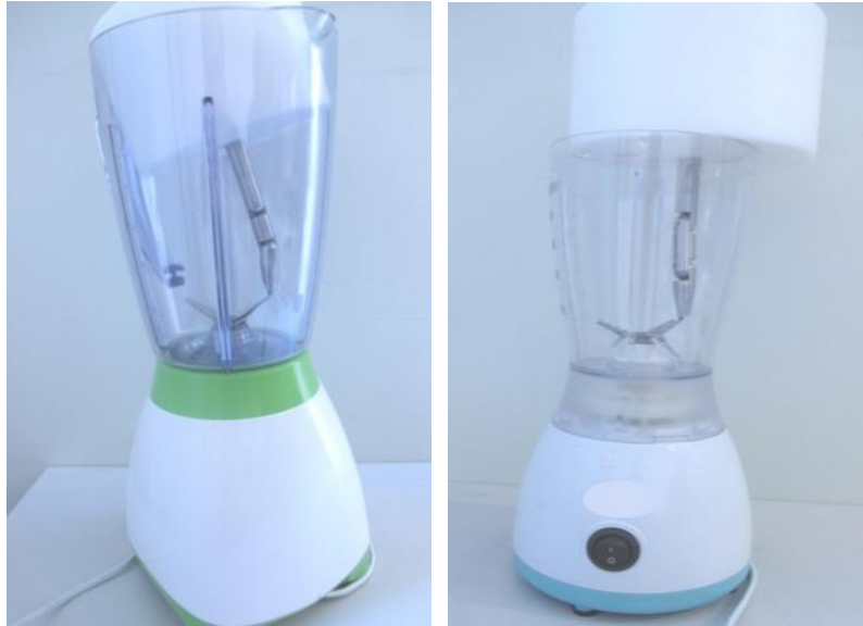
Figure 11 Access to rotating blades with test probe
