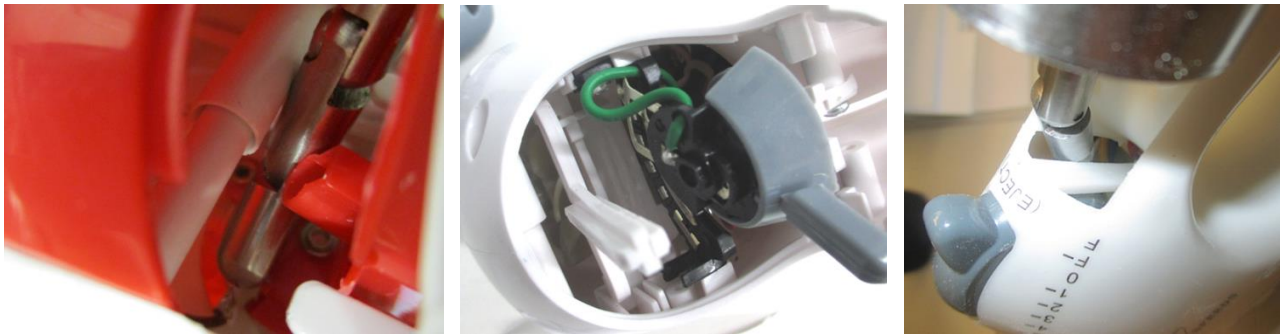
Figure 15 Accessible live parts after the standard drop test
