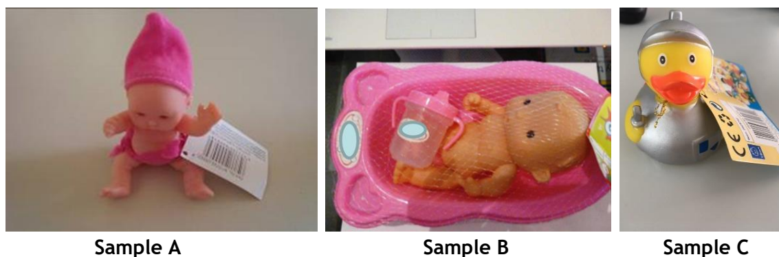
Figure 9 - Samples that failed the 'migration of BPA' test
